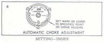
Loosen the three retaining screws and rotate the choke cover counter-clockwise against coil tension until the index mark is in line with the index point on the choke housing. At room temperature the choke valve should be lightly closed.
