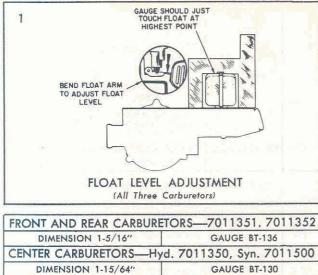
With the air horn inverted and the gasket in place, position the float level gauge over the float so it rests against the pump side of the power piston shaft, with the outer leg in line with the center of the float.
